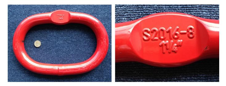
The photographs above show the overall size of the master link, and the part number embossed on the flat section
